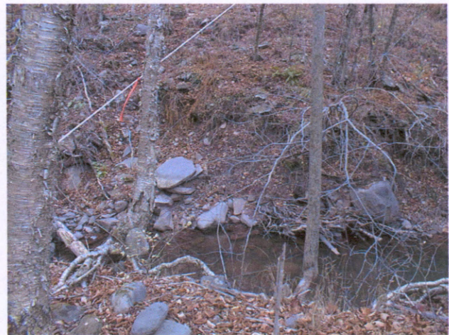
Photo 6. Eroding left bank at valley wall hillside, monitoring cross-section 18 (flow from left to right).
