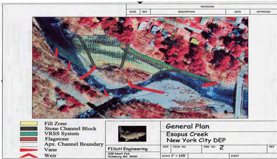
Figure 4. Original conceptual design. Final design is slightly different with changes in weir location and orientation and one rock vane moved just downstream of Woodland Valley.
