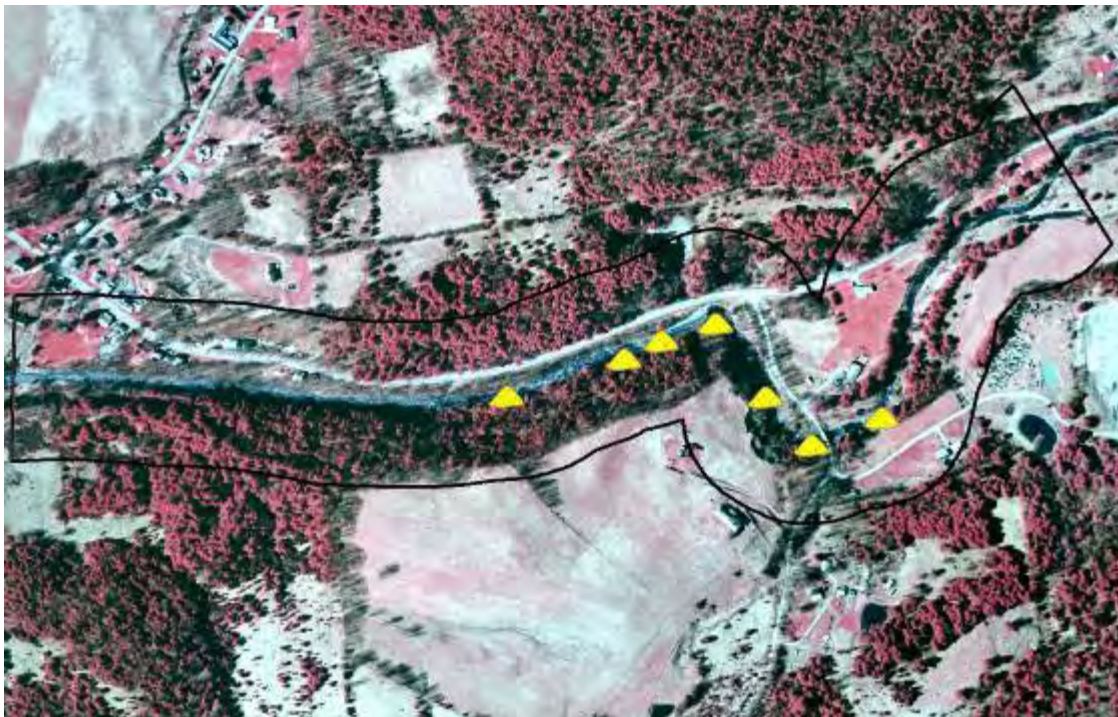
Figure 3.1.4. Example of the clay exposures (yellow) mapped during the Manor Kill 2008 stream feature inventory. This is Management Unit eight of ten and is located approximately 0.6 miles upstream of the Schoharie Reservoir.
