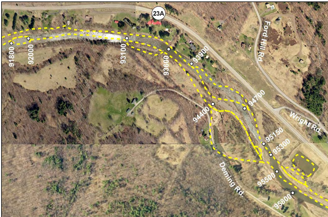
Wetland boundaries approximately delineated by NWI from Station 95800 to 91800
