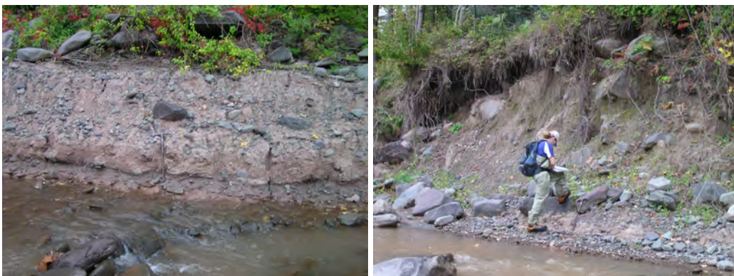
2.4.9 Examples of glacial till: (a) lodgment till and (b) melt-out till over lodgment till
