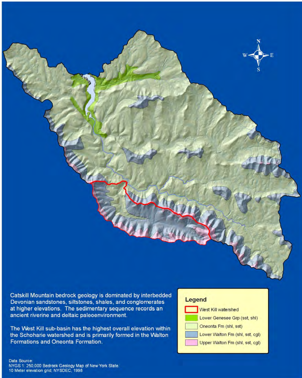
Figure 2.4.2 Bedrock geology of the upper Schoharie Watershed
