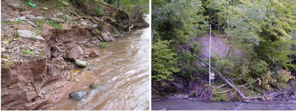
2.4.8 Glaciolacustrine silt/clay deposits in (a) stream bank and (b) hill slope failure on West Kill
