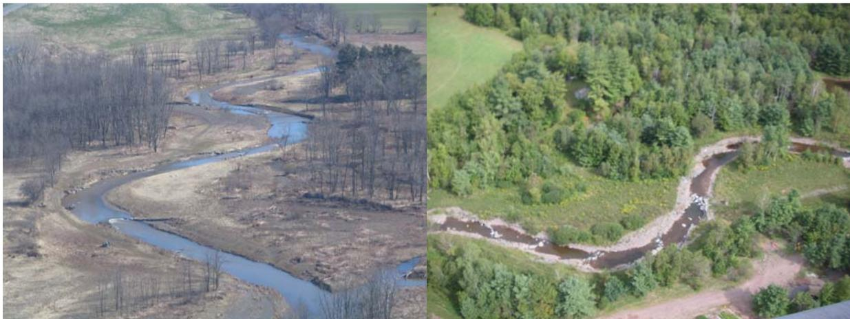
*Greene County streams after their meander geometry was restored to the extent necessary to move sediment and flow without excess erosion or deposition (bottom photos). The proper meander geometry is determined through detailed stream assessment. Also, a diagram showing the typical position of pools and riffles within a meandering stream, and a few other stream meander geometry patterns (top).*
