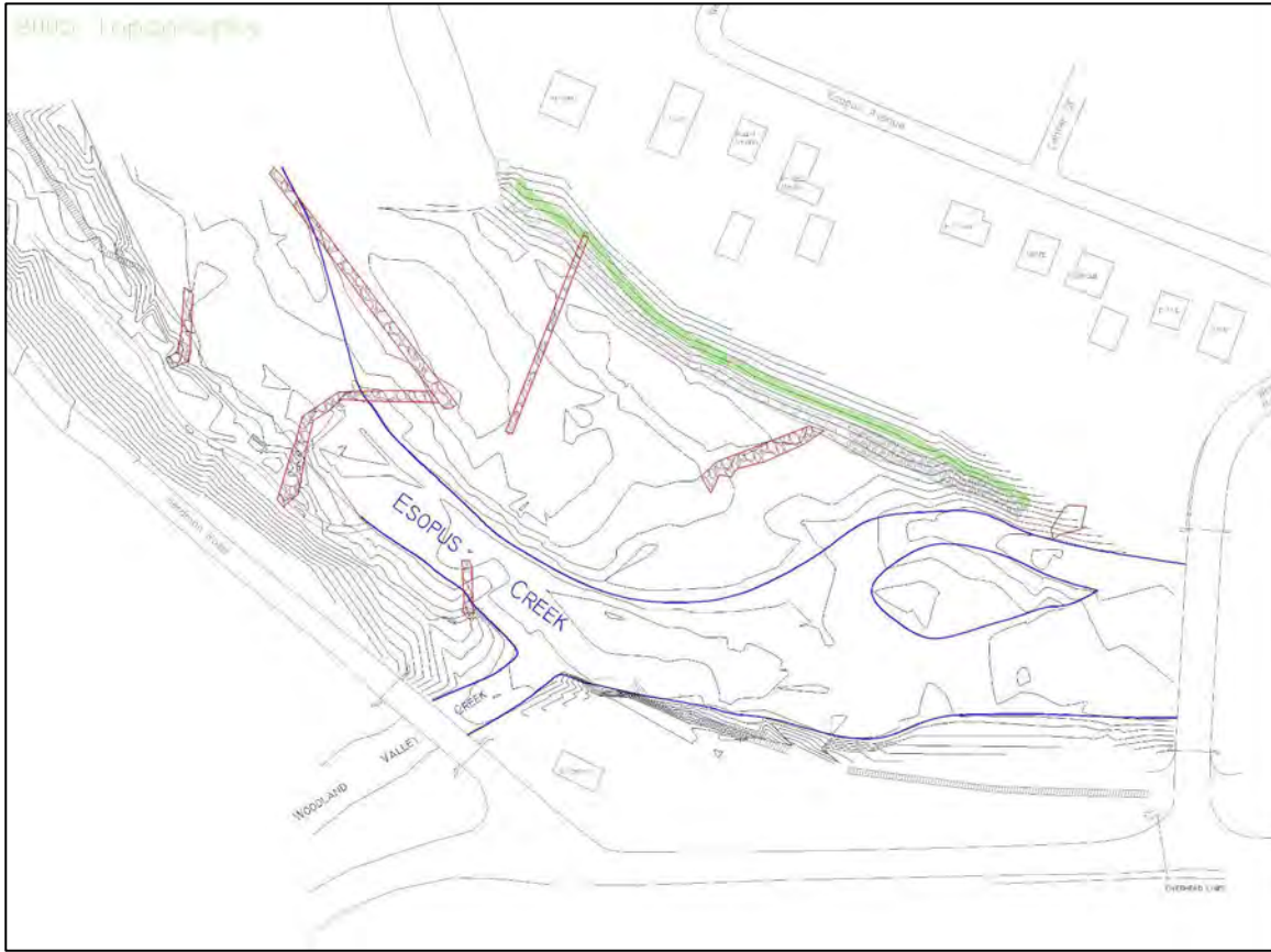
Figure 7. Post April 2005 flood topographic survey with schematics of remaining project features.
