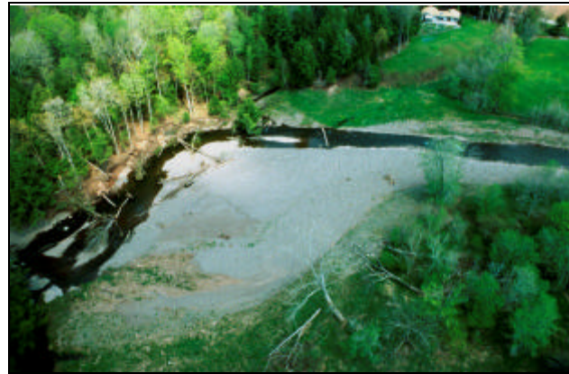
Image of excessive deposition and bar formation at the bottom of project reach.
