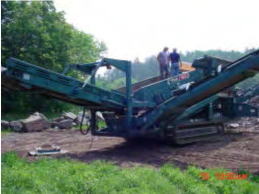
Figure 13: Gravel screen setup
