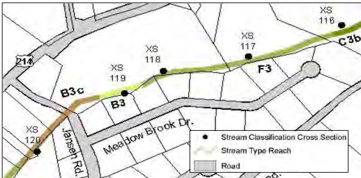
Figure 7 Cross-sections and Rosgen stream types for Management Unit 7
