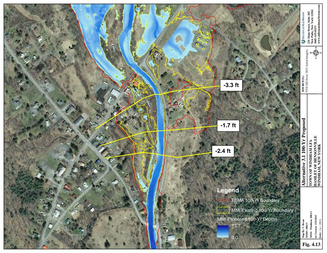
vertical walls and flows under the Route 23 (Main Street) bridge, which acts as a hydraulic constriction, causing extensive flooding along Mill Street. Combined with high backwater conditions in the Batavia Kill, floodwaters from Mitchell Hollow flow onto Route 23 and begin flowing west through Windham.
