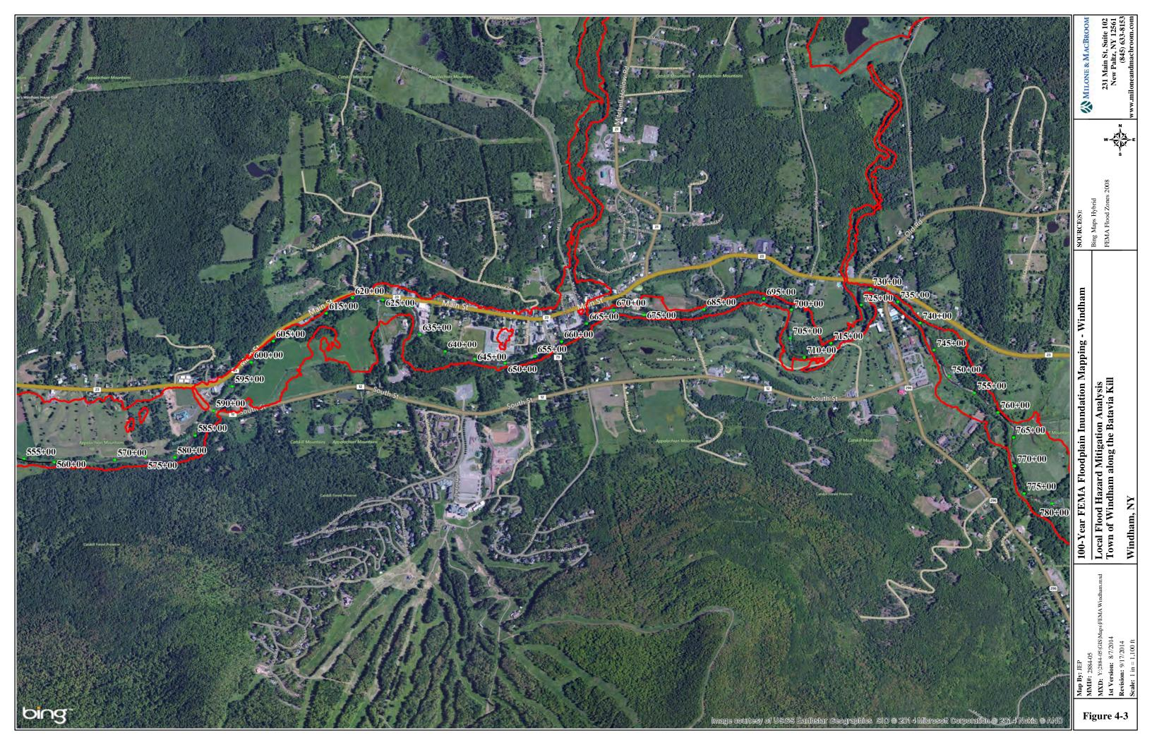
For purposes of water surface elevation computations, the model was run in subcritical flow regime, which will tend to use slower velocities but higher water surface elevations, and also provides the worst case scenario for flood surface elevations.
