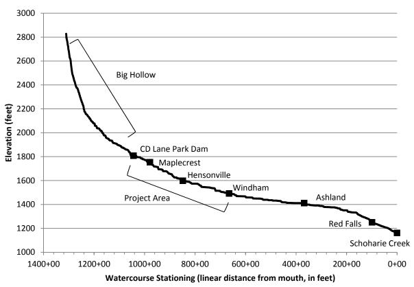
Flood profiles published in the FEMA FIS indicate that none of the bridges that span the Batavia Kill are inundated during the 100-year flood event. The 100-year flood event does bypass multiple bridges at the low lying areas on either side, including Slater Road (STA 967+00), Route 40 in Maplecrest (STA 937+50), Route 65 (STA 812+25), golf course bridge (STA 702+00), Route 79 (Church Street) (STA 658+25), and Route 12 (STA 590+00).
