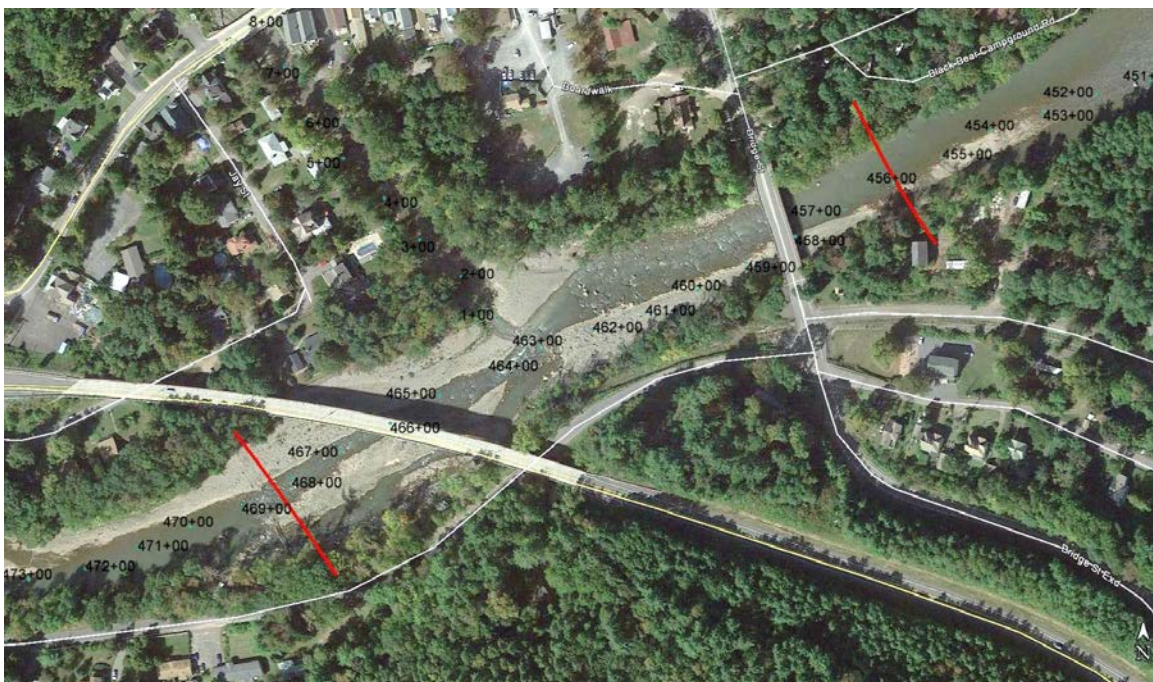
Figure 4-6 Location Along Esopus Creek Where Dredging of Channel Was Modeled
