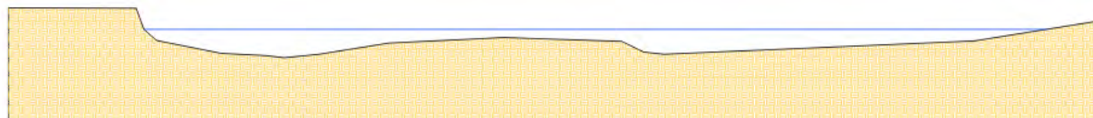
Figure VI-40: Cross section #4 at eroded bank on Valley View Farm, note the very high width to depth ratio.
