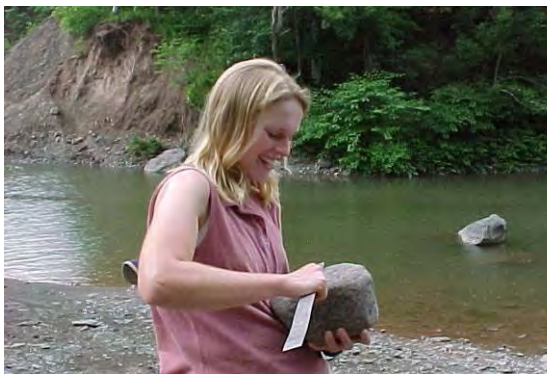
Figure 5 Measuring bed sediment particles
