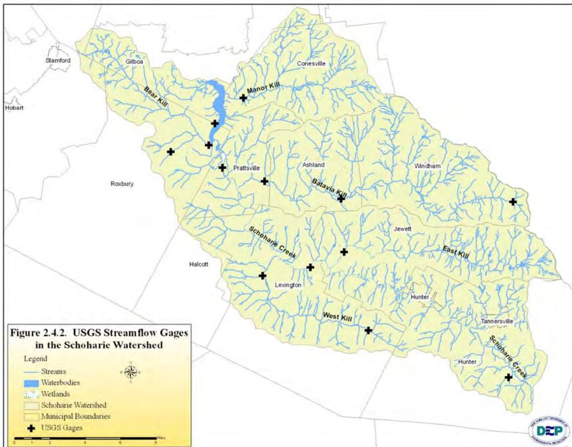
The United States Geological Survey (USGS) maintains two continuously recording stream gages on the Schoharie Creek near Lexington (established 1999, drainage area 96.8 mi<sup>2</sup>,
