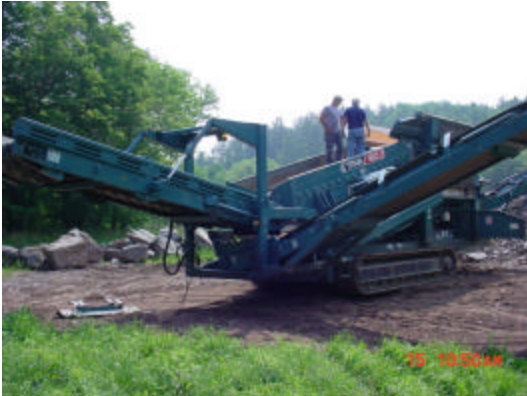
Figure 13: Gravel screen setup
