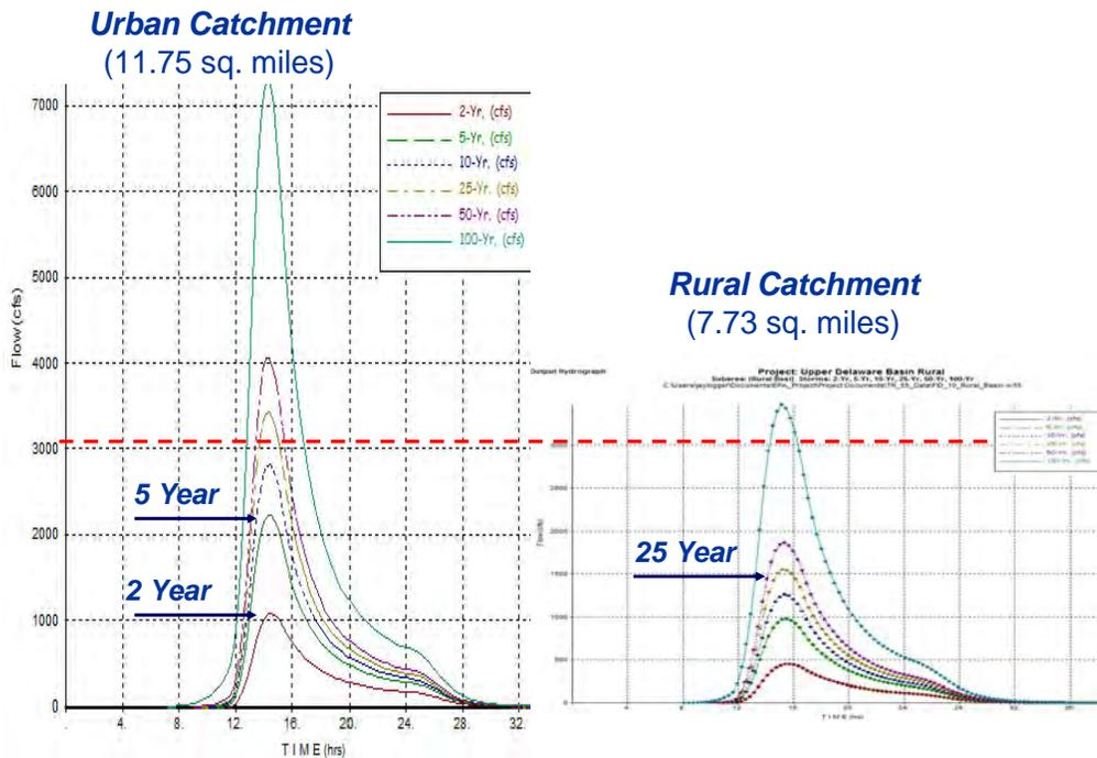
**Figure 37:** TR-55 Model Existing Stormwater Peak Discharges: Typical Rural and Urban Headwater Catchments. Note: the dashed red line indicates that the vertical axes from both hydrographs match up between 0 – 3,000 CFS.
