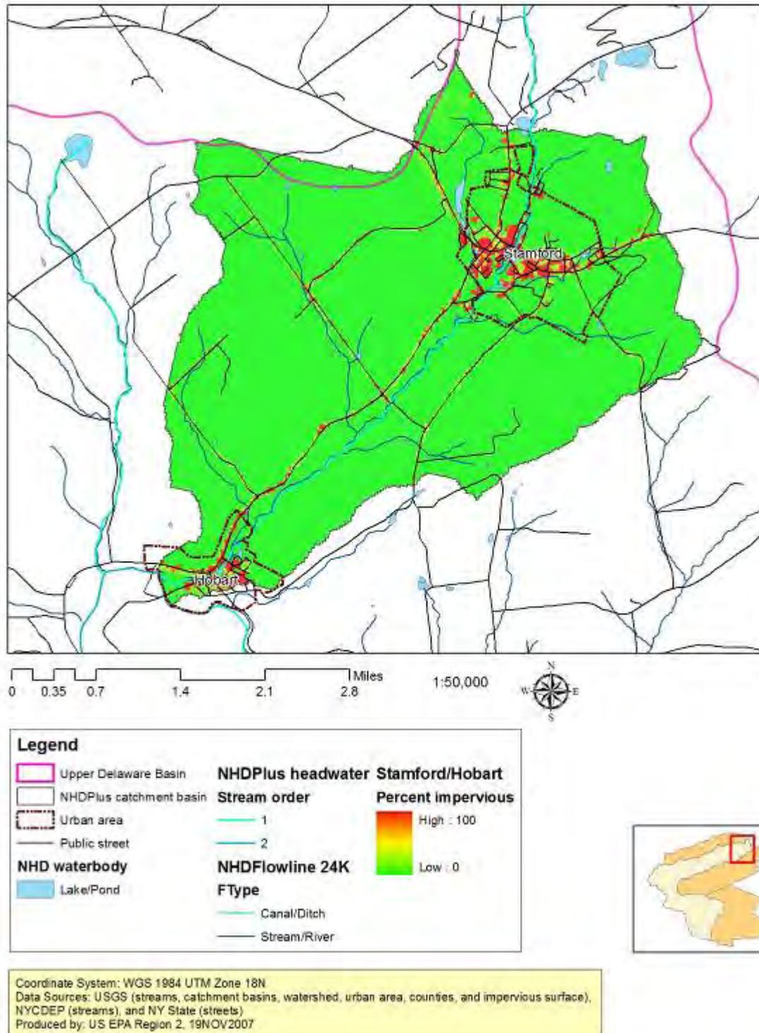
**Figure 31:** *Impervious Surface Model: Stamford-Hobart Headwater Catchment 2001:* the percent “red” in the Stamford-Hobart color-ramp indicates percent impervious surface cover (based on National Land Cover Data 2001).
