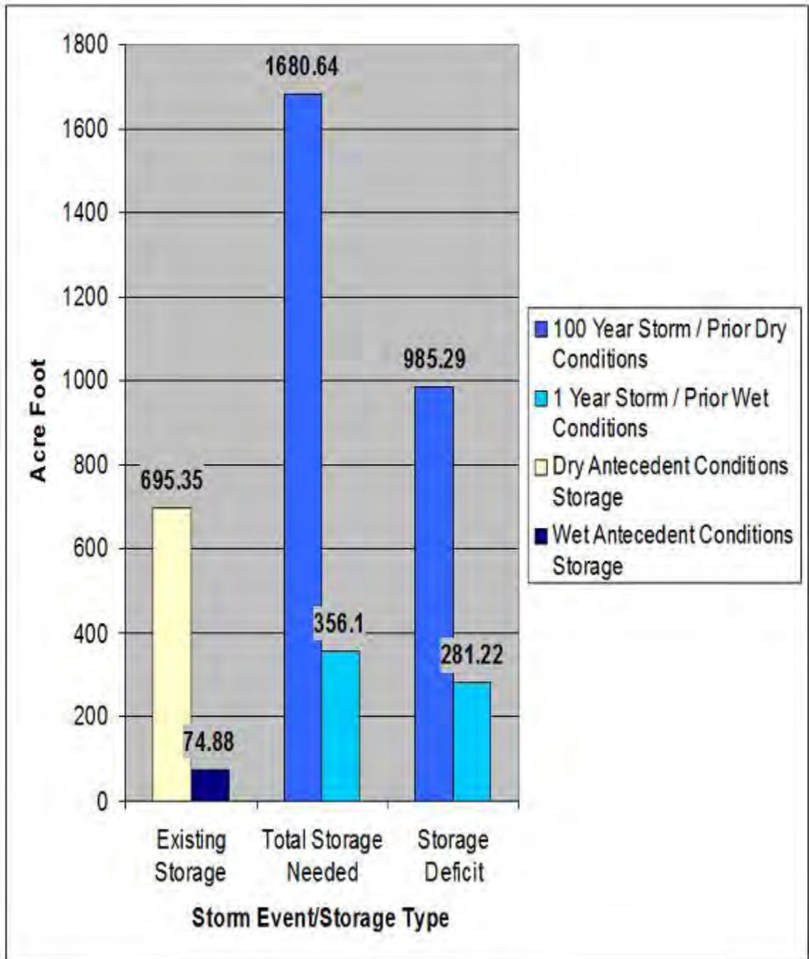
**Figure 47:** Wetland Surface Water Storage (1-Year and 100-Year, 24-Hour Storm Events): Urban Headwater Catchment. Note: the different storm events are based on the results from the Cirno, 2006 study.
