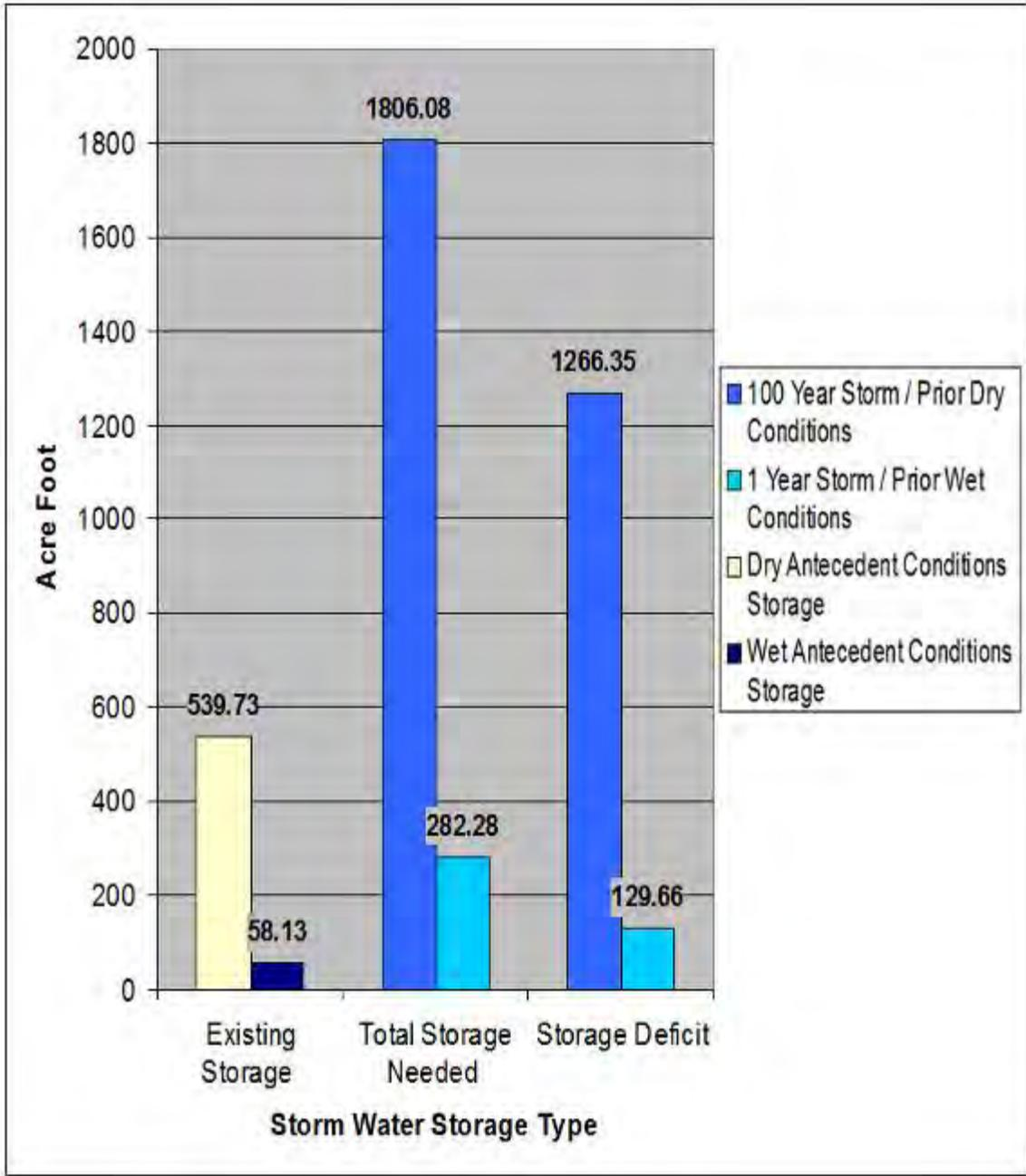
**Figure 44:** Wetland Surface Water Storage (1-Year and 100-Year, 24-Hour Storm Events): Rural Headwater Catchment. Note: the different storm events are based on the results from the Cirno, 2006 study.
