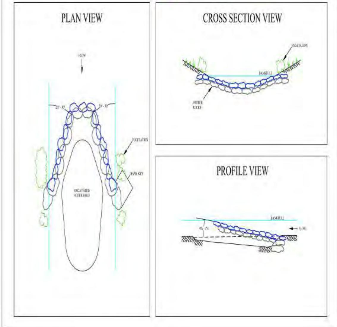
**Figure A.6: Typical Rock Cross Vane Structure Construction Drawing**
