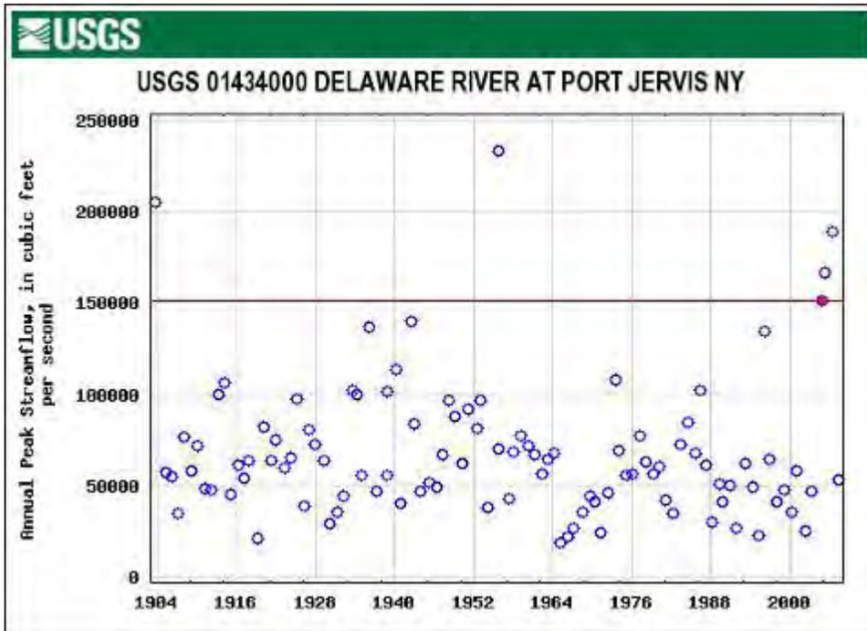
**Figure 26:** USGS 01434000 Delaware River at Port Jervis NY: peak annual stream flow at Port Jervis, NY (USGS, 2008). The read dot and line indicate the 90-year recurrence interval of the peak flow event of 2004 (Brooks, 2005).
