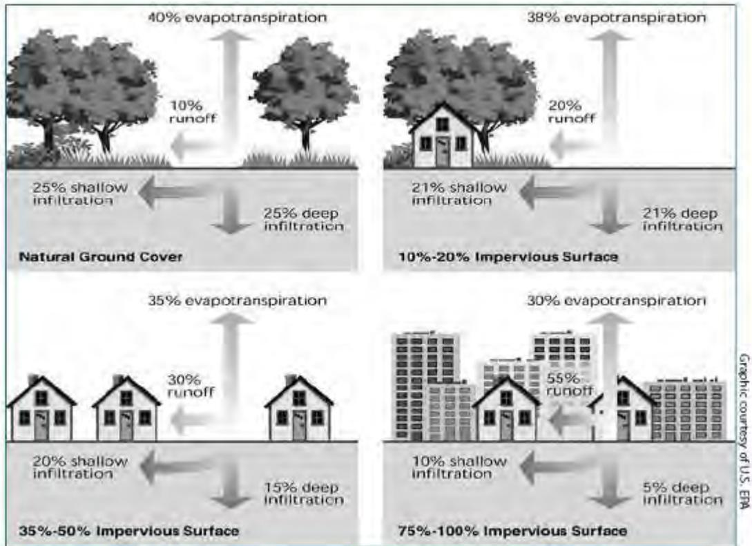
**Figure 56:** *Urban Development and Associated Stormwater Runoff Rates* (Richards, 2006).
