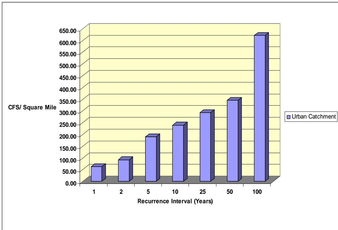
**Figure 83:** TR-55 Model 24-Hour Peak Discharge Rates per Square Mile: Stamford-Hobart Headwater Catchment. Note: the catchment size is 11.8 sq. miles.
