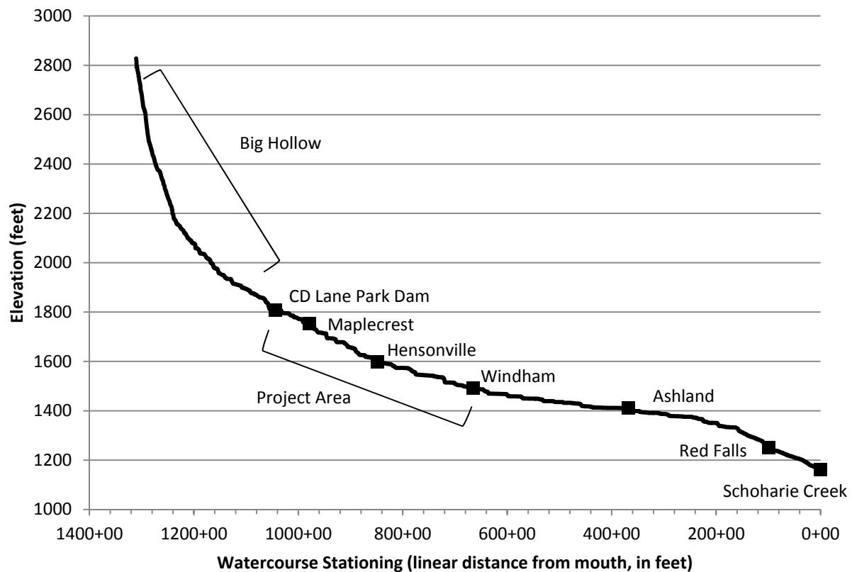
Flood profiles published in the FEMA FIS indicate that none of the bridges that span the Batavia Kill are inundated during the 100-year flood event. The 100-year flood event does bypass multiple bridges at the low lying areas on either side, including Slater Road (STA 967+00), Route 40 in Maplecrest (STA 937+50), Route 65 (STA 812+25), golf course bridge (STA 702+00), Route 79 (Church Street) (STA 658+25), and Route 12 (STA 590+00).
