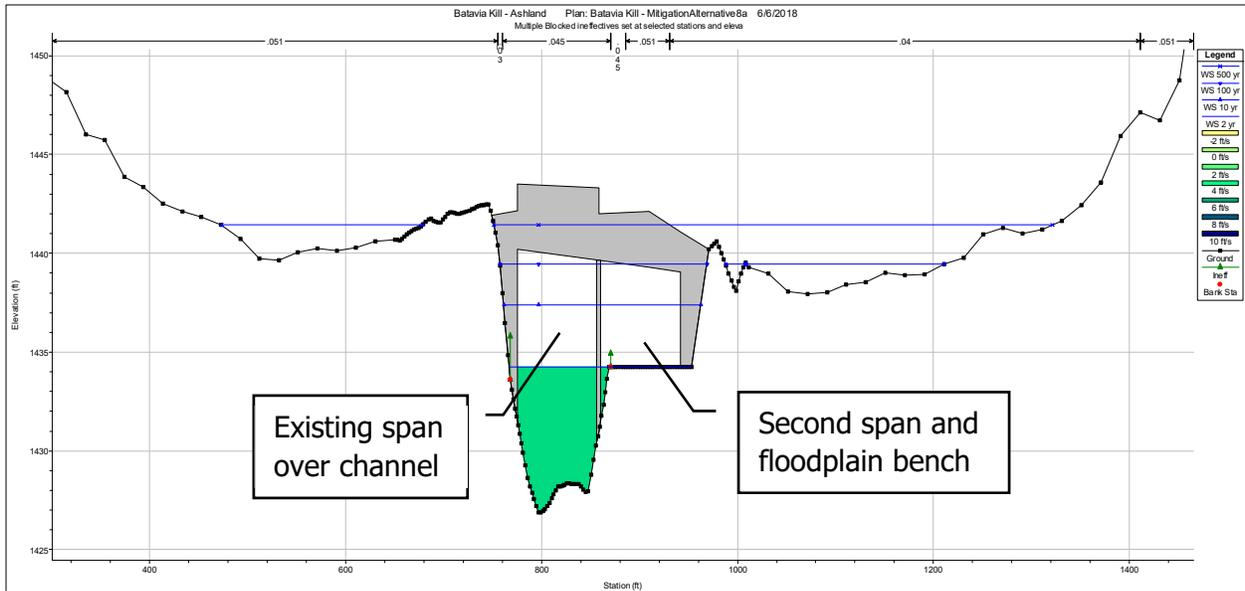
**Figure 4-4: Representation of Alternative 5 in Hydraulic Model**
