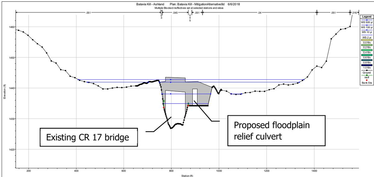
**Figure 4-3: Representation of Alternative 4 in Hydraulic Model**
