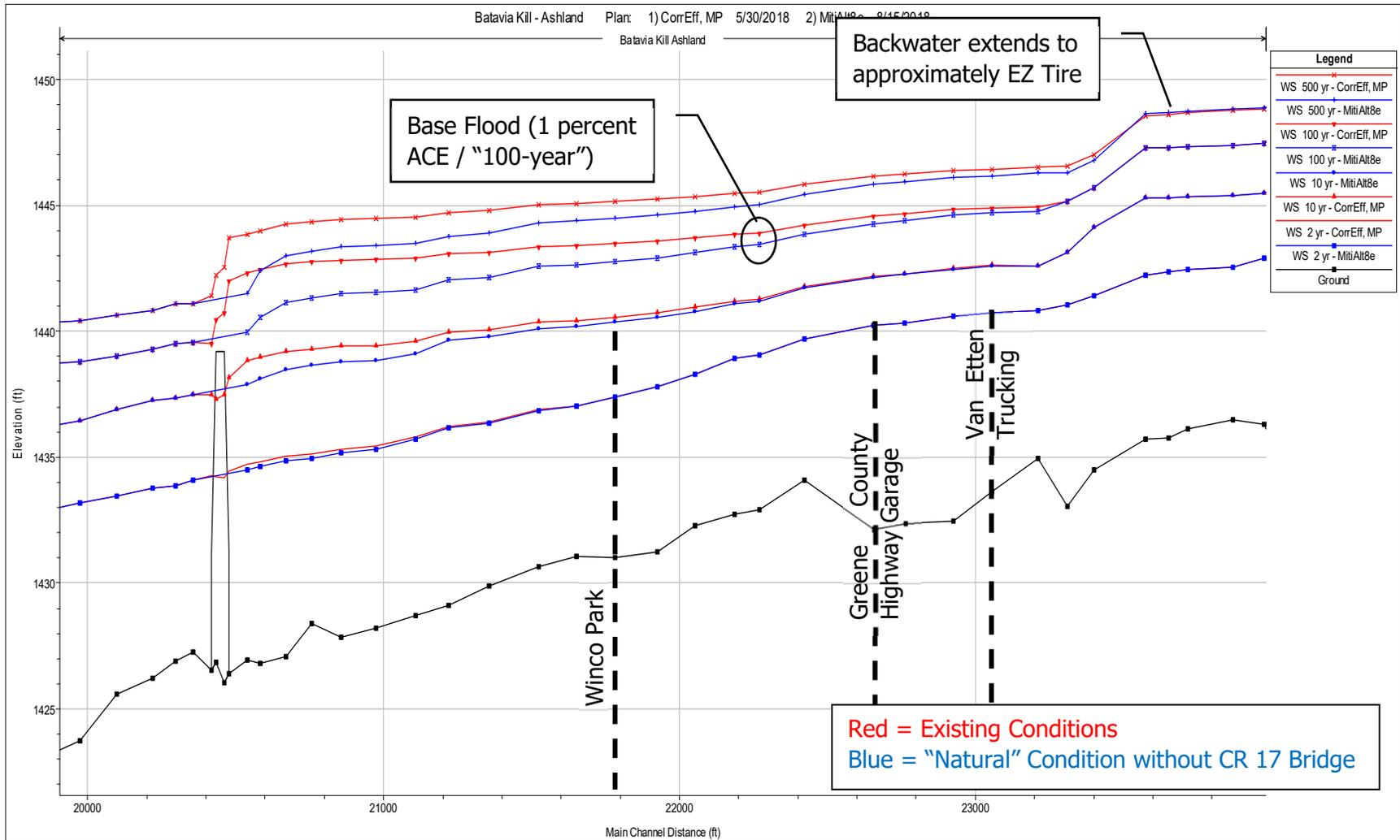
**Figure 4-1: Comparison of Corrected Effective Model at County Road 17 to Theoretical "Natural Condition" Model without Bridge**
