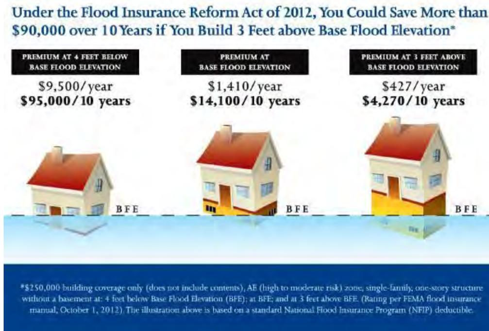
**Figure 4-6: Infographic of Structure Elevation; Source: FEMA**
