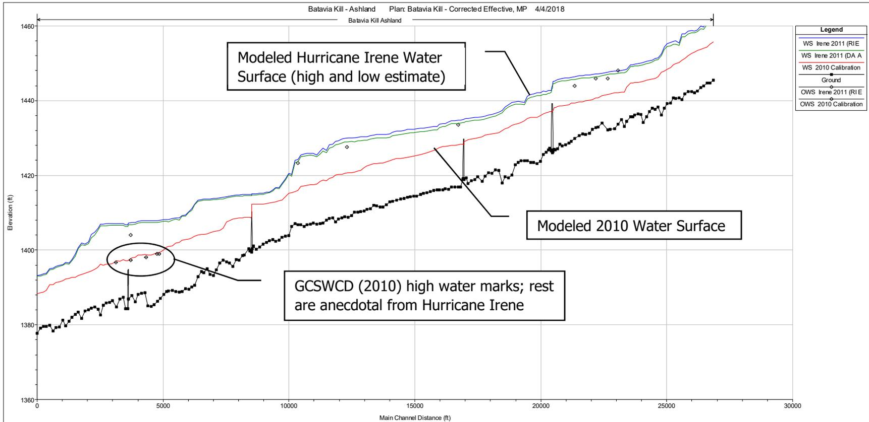
**Figure 3-7. Comparison of Corrected Effective Model to Observed High Water Marks**
