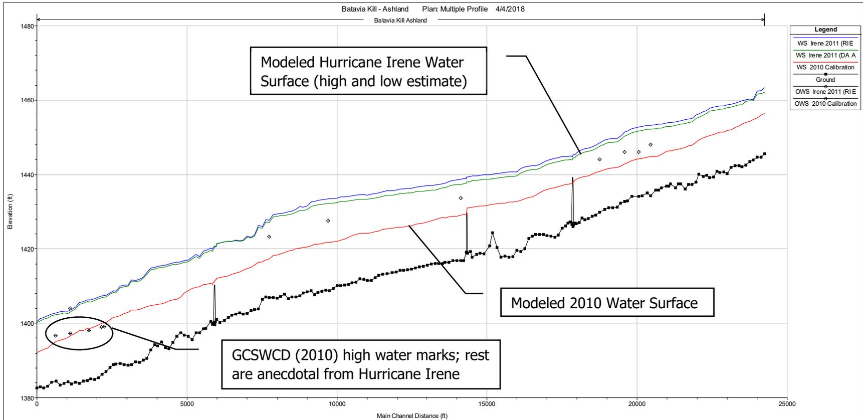
**Figure 3-6. Comparison of Duplicate Effective Model to Observed High Water Marks**
