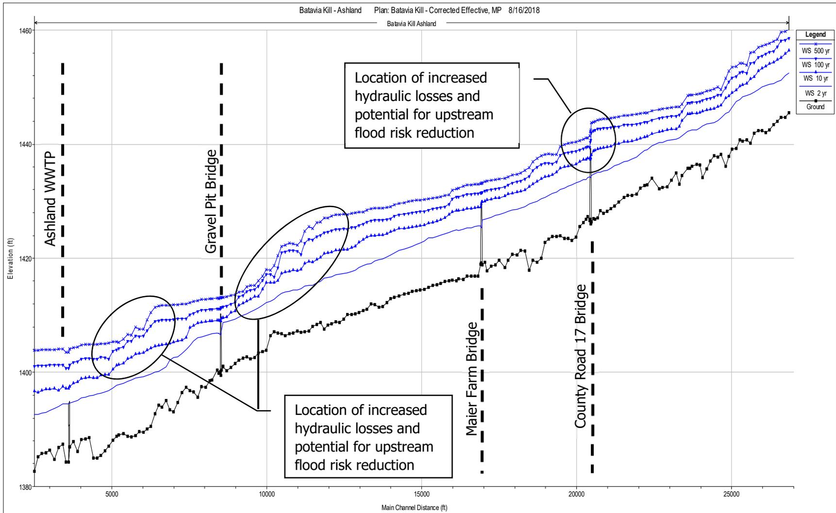
**Figure 4-5: Corrected Effective Model Results and Locations of Increased Hydraulic Losses**
