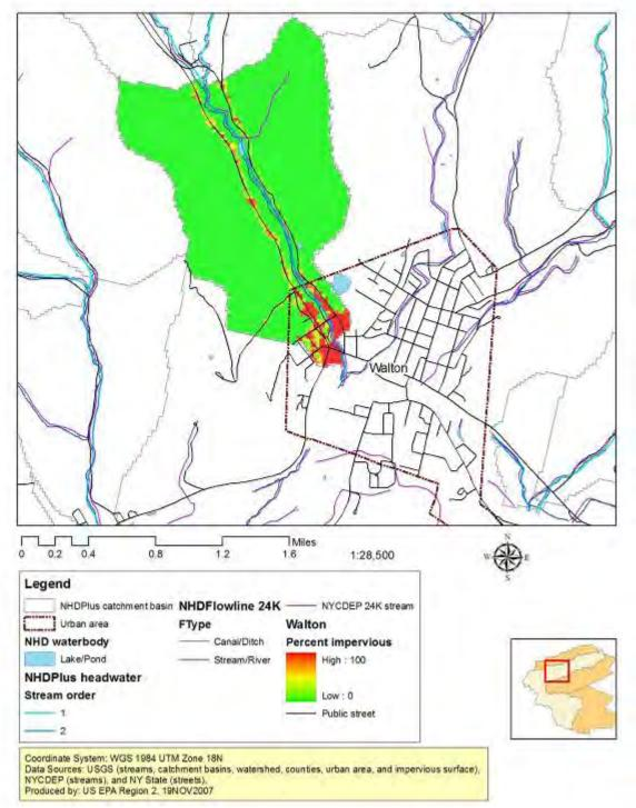
**Figure 30**: *Impervious Surface Model: Walton Headwater Catchment 2001*: the percent "red" in the Walton color-ramp indicates percent impervious surface cover (based on National Land Cover Data 2001).
