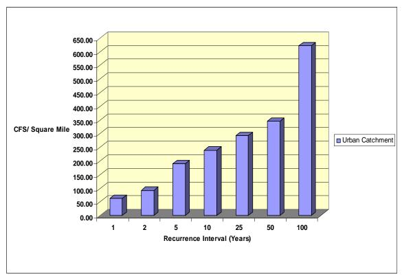
**Figure 83:** *TR-55 Model 24-Hour Peak Discharge Rates per Square Mile: Stamford-Hobart Headwater Catchment.* Note: the catchment size is 11.8 sq. miles.
