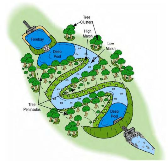
Figure 58: Wooded Stormwater Wetland (Cappiella et al., 2008).
