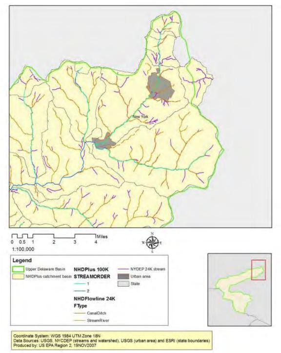
**Figure 25:** *Upper Delaware Basin: Close-Up View of Headwater Streams, Delaware County, NY:* view of the northeast portion of the watershed. Note the difference in the number of stream flowlines between the 1:100K and 1:24K stream networks.
