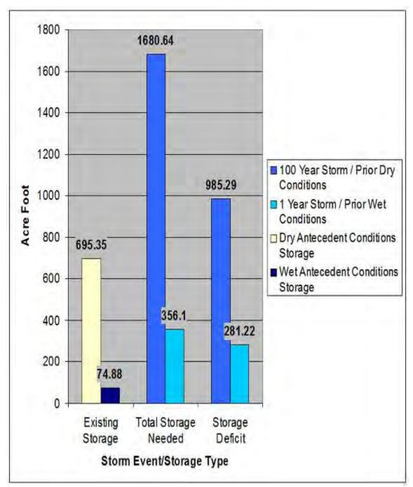
**Figure 47:** Wetland Surface Water Storage (1-Year and 100-Year, 24-Hour Storm *Events*): Urban Headwater Catchment. Note: the different storm events are based on the results from the Cirmo, 2006 study.
