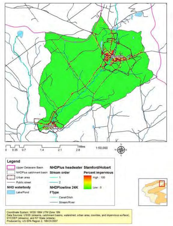
**Figure 31**: *Impervious Surface Model: Stamford-Hobart Headwater Catchment 2001:* the percent "red" in the Stamford-Hobart color-ramp indicates percent impervious surface cover (based on National Land Cover Data 2001).
