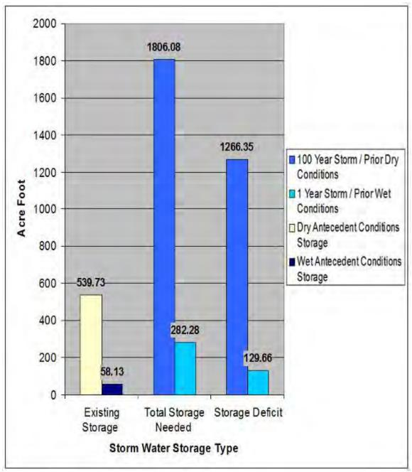
**Figure 44:** Wetland Surface Water Storage (1-Year and 100-Year, 24-Hour Storm *Events*): Rural Headwater Catchment. Note: the different storm events are based on the results from the Cirmo, 2006 study.
