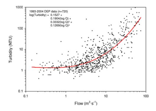
Figure 3.9. Relationship between streamflow and turbidity for Esopus Creek at Allaben. (R. Gelda, personal communication, 2007)
