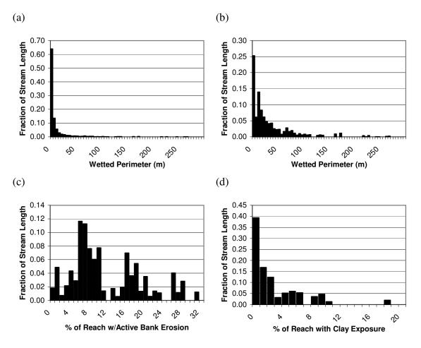
Figure 3.4. Histograms of indicators of sediment supply: (a) wetted perimeter including all streams; (b) wetted perimeter only including  $3^{rd}$  order and above streams; (c) percent of reach with active bank erosion and (d) percent of clay exposures.
