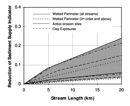
Figure 3.7. Envelope of reduction of in-channel sediment supply indicator versus length of stream based on the cumulative distributions of indicators from Figure 3.6 with 20-80% reduction efficiency.
