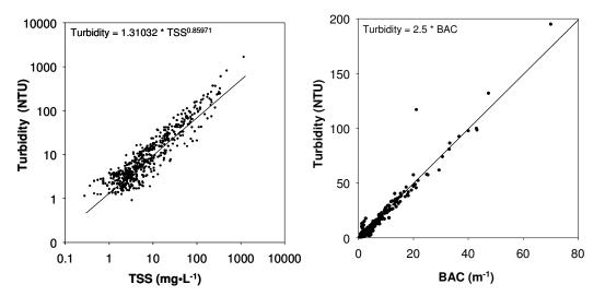
Figure 3.8. Relationships used to relate suspended sediment to turbidity (R. Gelda, personal communication, 2007) and beam attenuation coefficient (Effler et al., 2006).
