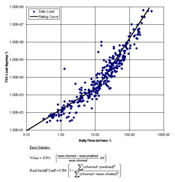
Figure 3.2. Rating curve showing relationship between suspended sediment load and daily flow for USGS streamflow gage located at Schoharie Creek at Prattsville. Error statistics show a good fit with % bias of -0.9% (Thomann, 1982) and Nash-Sutcliff coefficient of model efficiency of 0.784 (Nash and Sutcliff, 1970).
