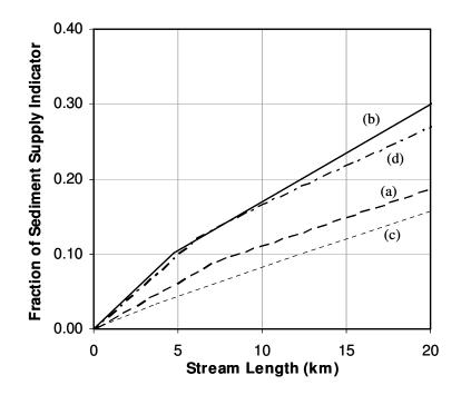
Figure 3.6. Cumulative distribution of indicators of sediment supply based on stream length: (a) wetted perimeter including all streams; (b) wetted perimeter only including 3<sup>rd</sup> order and above streams; (c) percent of reach with active bank erosion and (d) percent of clay exposure
