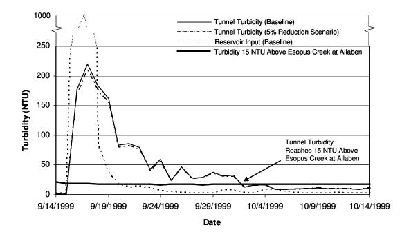
Figure 3.12. Example time series of model output showing storm input turbidity and resulting modeled tunnel turbidity for base case and 5% reduction scenario.
