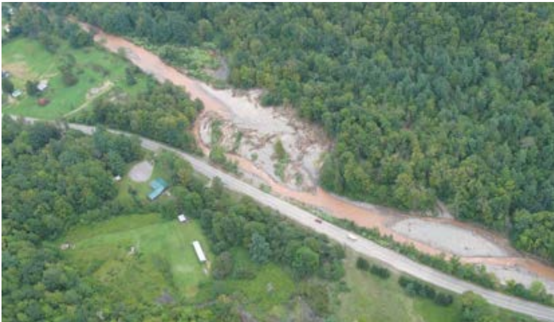
Photo 3-2 Large wood accumulation and lateral channel adjustment along flood-prone section of NY-214 after Tropical Storm Irene in 2011. Photo provided by NYCDEP SMP.
